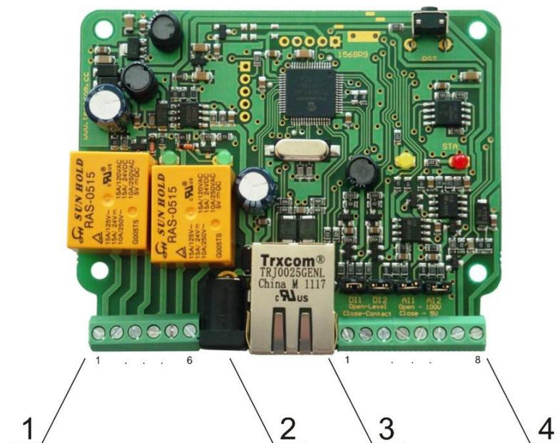
**Connector 1** – 6-pin connector pinout is shown in the table below:
