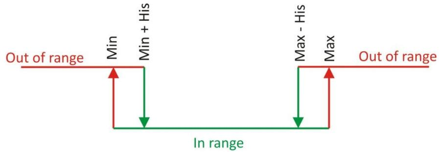
For analog input similar range can be set. It is mandatory that chosen range correspond with the range selection jumper J1 - 0÷5VDC (close) or 0÷100VDC (open).
